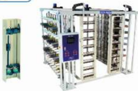
CENTRALLY AUTO TENSION CONTROLLED CREEL
